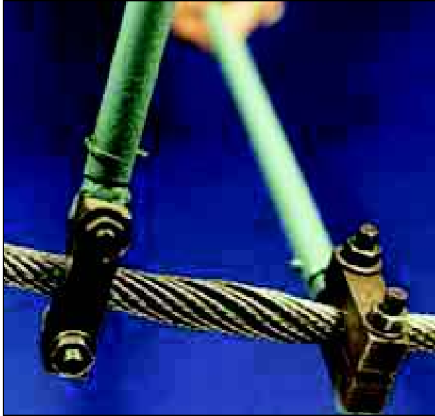
Figure 13. Internal examination of wire rope (Source: Certex)
