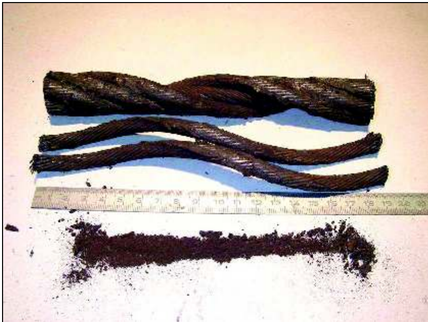
Figure 10. Wire Rope specimen with two separated strands showing the level of corrosion product found within the rope during de-stranding.
