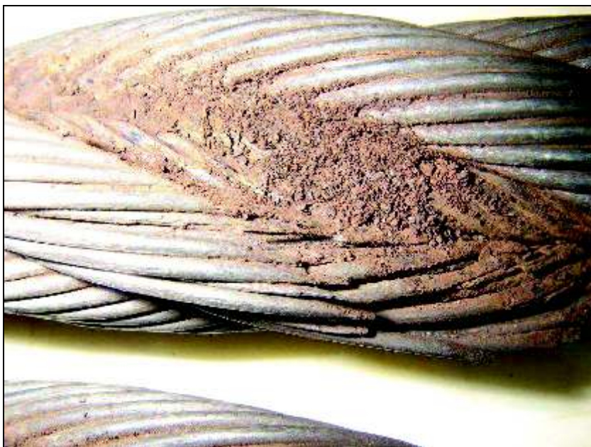
Figure 8. Wire breaks located next to each other in the outer strand of the wire adjacent to the points of failure with evidence of acute corrosion.
