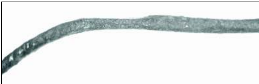
Figure 12. Abrasion on a contact point on an outer wire of the core strand of the steel core.
