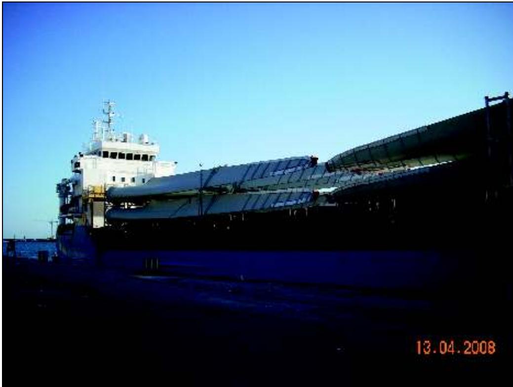
Figure 1. Cimbris (hatch cover gantry crane is shown in its aft stored position)
